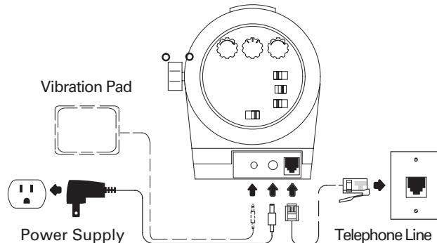
**Important:** To connect the alarm clock to a telephone connection for use as a signal amplifier, you may need an appropriate adapter.
