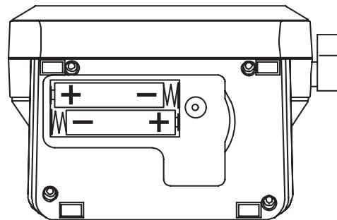
**Important:** Pay attention to correct polarity when inserting the batteries.
