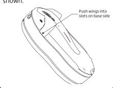
To remove the clip press one of the wings away from the body. Do not try to remove the clip by lifting the clip away from the battery cover as you may damage the parts.
