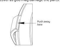
To install the neck cord remove belt clip and thread the cord as shown, and replace the belt clip. The neck cord has a safety release feature to avoid you getting trapped by the cord.
