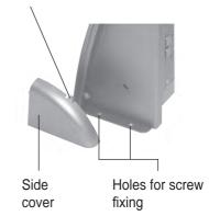
Press on the retaining clip and remove the cover.
