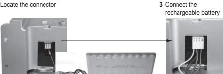
4 Place the rechargeable battery in the battery compartment
